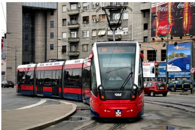
**Figure 1:** Picture of CAF Urbos 3 electrical multiple units operating on of Belgrade Urban Line
