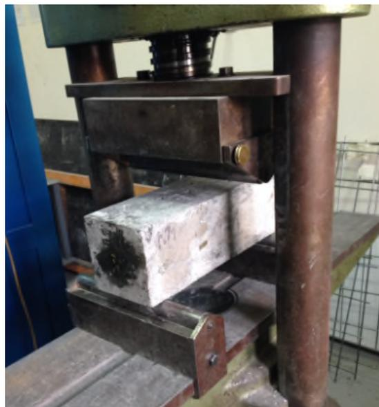
Figure 5: Testing of the flexural strength
