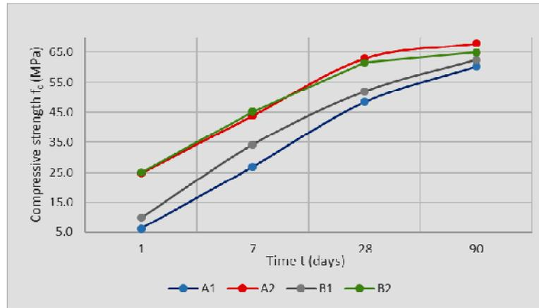
Figure 4: Compressive strength vs. time up to 90 days
